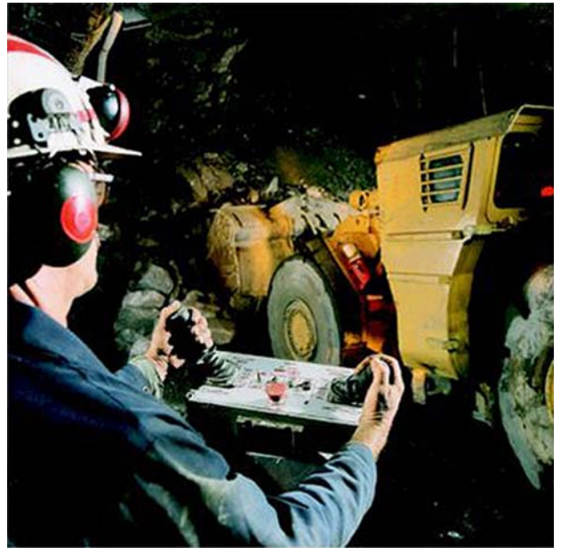
Underground communication and radio remote control systems for mining applications
